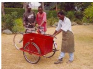
In order to increase the carrying capacity of a bicycle a side trailer was made. This uses only one extra wheel compared with a two wheeled trailer and bicycle wheels are costly.
