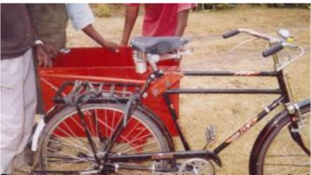
The trailer box was clamped to the bicycle in two places allowing it to be removed easily.
