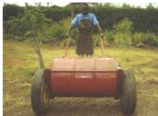
Where water transport is a major need this specialized water cart has a place. The 200 litre drum acts as the axle. The wheels and stub axles are held by the ½" pipes.
