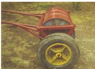
The wheel rim is rolled in a hand press then jig welded. The inner ring is welded to the rim.
